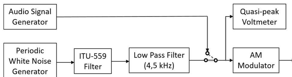
NOTE: The low pass filter has a cut-off frequency of 4,5 kHz and a minimum roll-off of 60 dB/octave.
