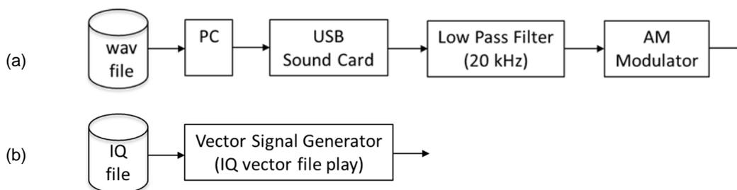
NOTE: The low pass filter has a cut-off frequency of 20 kHz and a minimum roll-off of 40 dB/octave.
